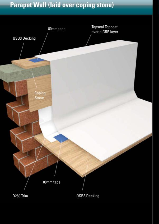
**Completed Parapet Wall** Laminate can be bonded to either the decking or pre-formed GRP profiles 'A' Type trim used on the the outer edge of the parapet wall
