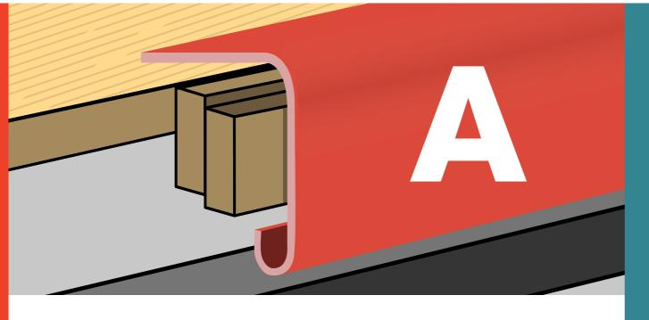
The 'A' type trim is a Drip Trim, fitted to the lowest edge of the roof to allow the rainwater flow into the gutter.
